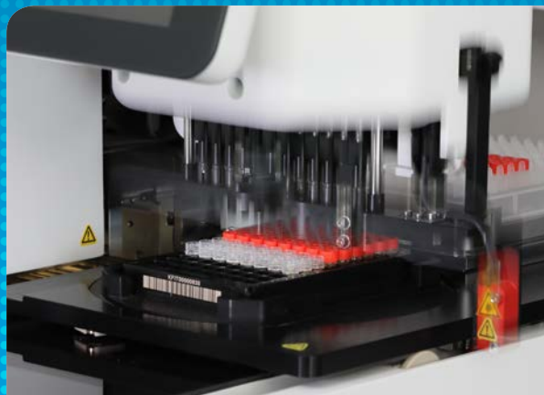
Fully-automatic 12 Channel Capper / Decapper
